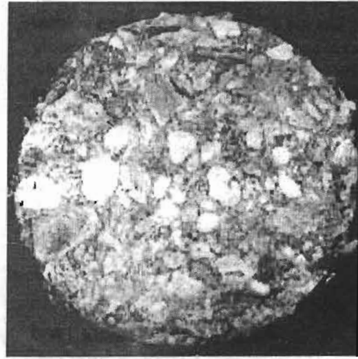
Photo 9: cross-section of specimen with big amount of polypropylene fiber, PP2 type.
